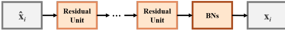
Figure 4. The refiner network. The tensor size remains the same throughout the network.
